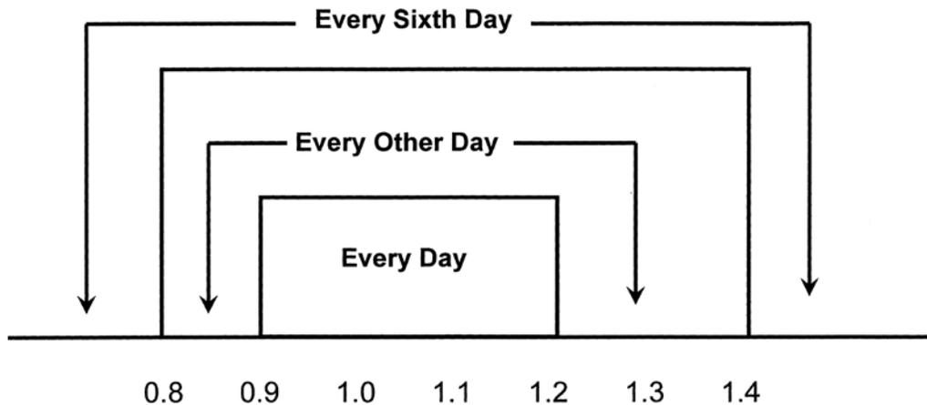
Figure 6.2 Sampling schedule based on ratio to the 24-hour PM<sub>10</sub> NAAQS
