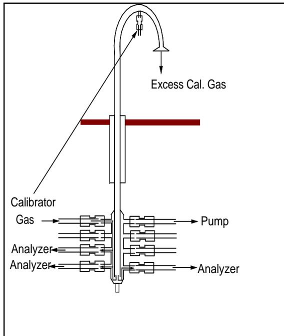
**Figure 7.4 Positions of calibration line in sampling manifold**
