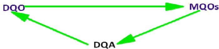
The DQO process functions to identify the allowable population and measurement uncertainty for a given objective. The monitoring program is then developed and quality control samples are identified and implemented
