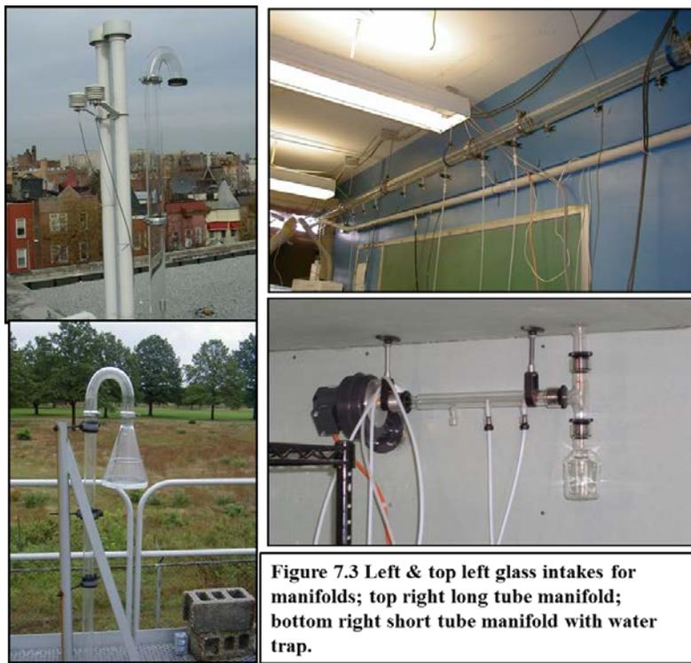
Figure 7.3 Left & top left glass intakes for manifolds; top right long tube manifold; bottom right short tube manifold with water trap.
